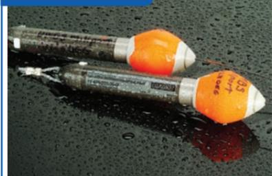
Satellite tracking tags such as the pair shown above cost US\$2,000 each. Their signal is picked up by orbiting satellites, and they record light, temperature and depth, as well providing information about how often the sharks return to the Seychelles, migration patterns and the diving habits and environment of the sharks. The information cannot be sent or received unless the tag breaks the surface and the satellite is visible.
